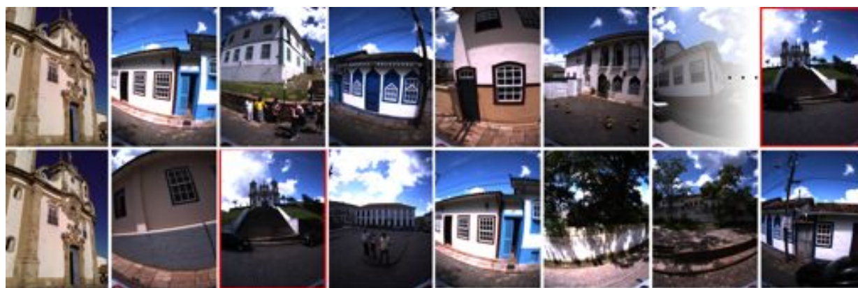
Fig. 1. Improvement of image matching by using subspace clustering: the first line shows normal matching where the query (first left image) is matched with the 209 th (last image) returned database image. After our method, at the second line, query image (first left image) is recognized as the 2 nd (third image) returned database image.
